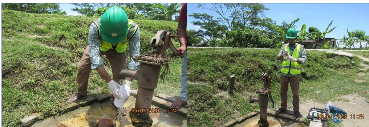
Sample Photographs of Groundwater Sampling Activities
