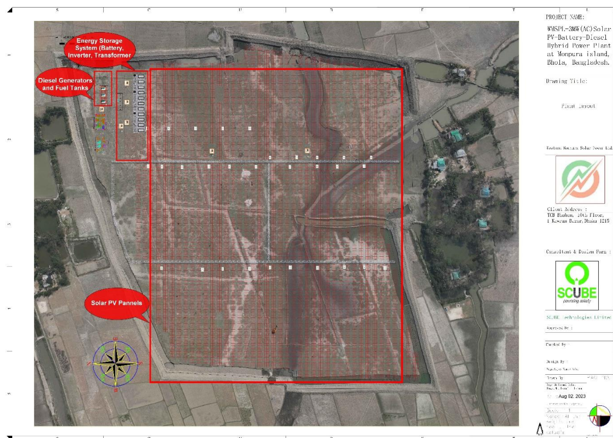
Figure 3-5: Plant Layout Showing Solar PV, Battery, and Diesel Generator Locations (source: WMSPL)
